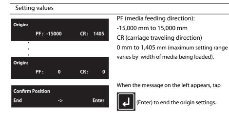
The arrow mark on the origin label shows the current print start position in CR direction.
