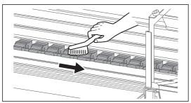
Brush off dusts on the pressure rollers with a soft brush.
