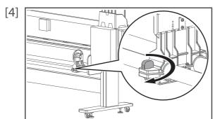
Twist the knob bolt on the right side of the media holder clockwise to tighten.
