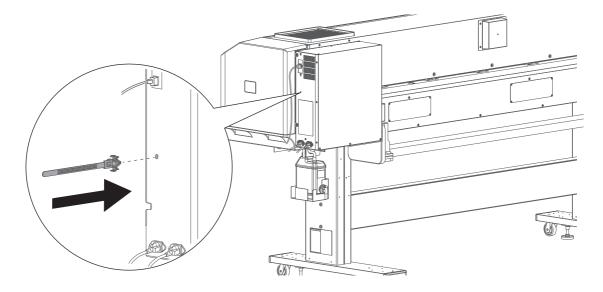
$[3] \qquad \text{Use the cable tie to secure the Ethernet cable to the printer.}$
