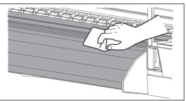
Use a soft cloth or paper towel slightly dampened with ethanol to clean off the ink on the platen, media guide and edge holders.
