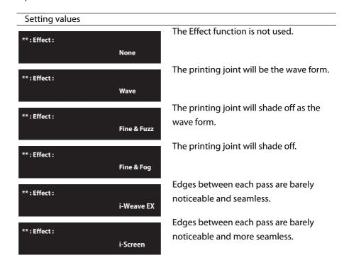
Type \*\*: 2 Adjust Print Sets up when adjusting the printer for the optimum quality of image print. Before adjusting this setting, enter the thickness of the media.
