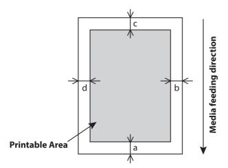
a=5 mm \*1 b=5 mm to 25 mm \*2 c=5 mm d=5 mm to 25 mm \*2
