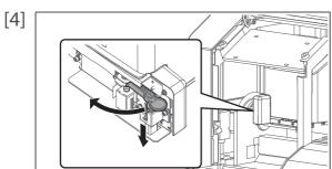
Press the cutter cap lightly, turn Cutter holder in the direction as illustrated below.
