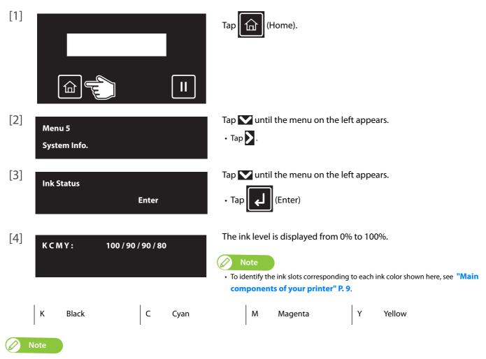
• If it is blinking at 10%, smartchip recovery is being performed on the corresponding S/C card.
