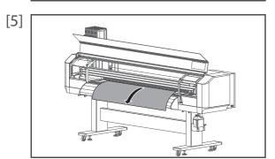
From the front side of the printer, pull the media for approximately 1 m.
