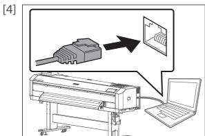
Connect the Gigabit Ethernet cable to the computer.
